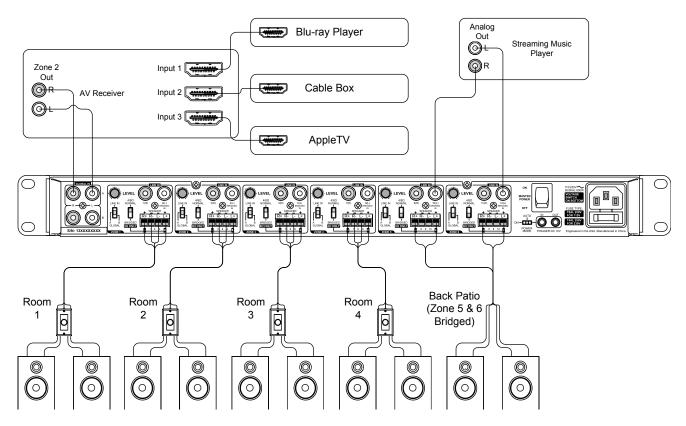
The diagram above illustrates the basic setup of a multi-room audio system with dedicated source inputs. See the notes below to understand the setup:
