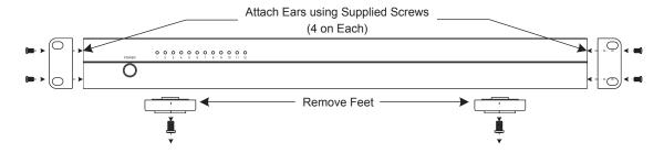
To mount the amplifier in the rack, 1-U of space is needed for placement, and 5 inches above the space should be left open to allow for adequate ventilation. Install the amplifier so that the rear of the unit can be accessed for connections and adjustments for the output zone.
