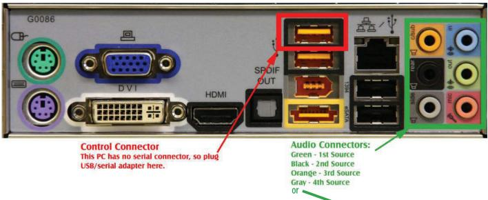
Back of typical PC, showing connector panel
